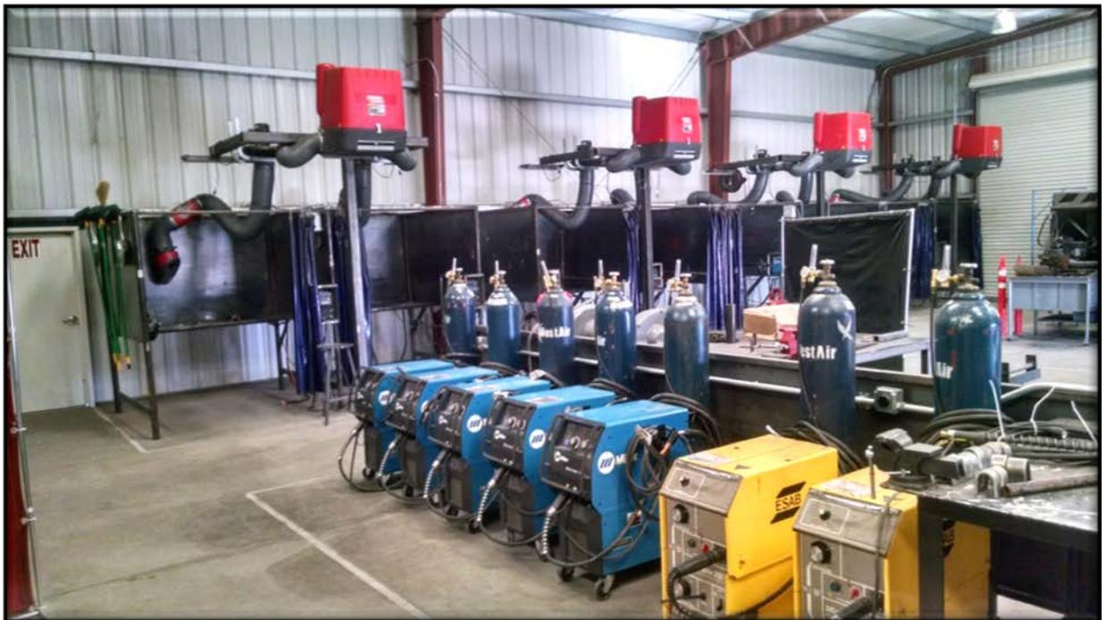
Welding booths with ventilation hoods and multiuse inert gas welders in the new welding facility
